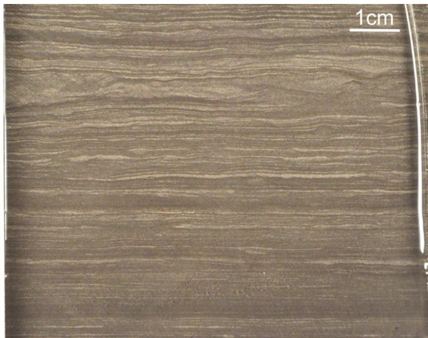
Figure O-06-3. Heterolithic lamination at 1628.9 m MD.
